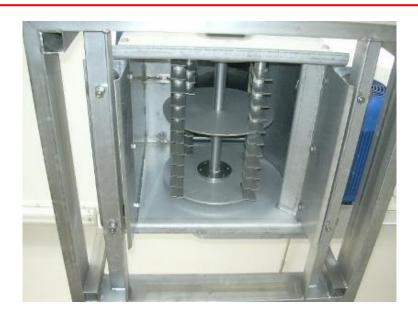
Machine suitable for chopping the stalks reducing up to 80% volume for storage during the harvest. The high number of revolutions of the machine allows to shred even small branches and other plant components discarded. The reception takes place by gravity from specific belt feeder or auger. Constructed entirely of stainless steel AISI 304, it has a roller movable knives with specific shape.
